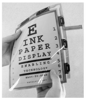
This flexible electronic paper display was created by E Ink Corporation and LG.Philips LCD in 2005. *Photo courtesy of LG.Philips LCD*.
