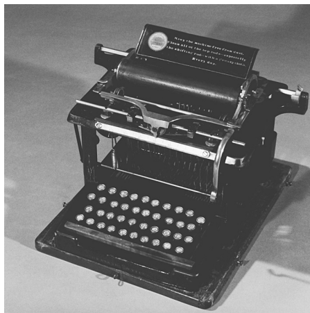
Remington 2 typewriter, circa 1880. This typewriter was the first of its kind to have upper- and lowercase letters. The space bar is made of wood. Newseum collection/ Courtesy Newseum.
