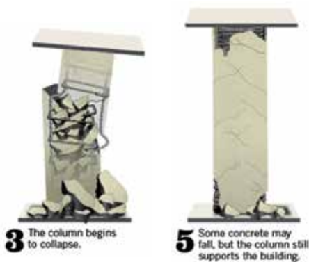
A graphic in the Los Angeles Times’s “Concrete Risks” illustrates the value of steel reinforcement in concrete buildings
